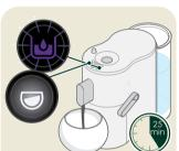
The cleaning key of flashes purple and the espresso key lights up, the descaling process starts.
