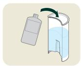
▶ Use descaler (0.5 I mixture) according to the manufacturer's instructions and fill the water tank.
