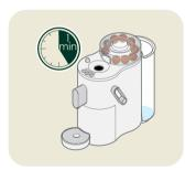
When the coffee machine is not used for 1 minute or the cleaning key (a) is pressed for 3 seconds, the coffee machine switches to energy-saving mode.
